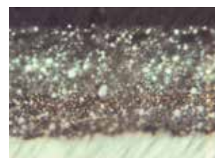
Gold particles in between the two layers of epoxy paint
